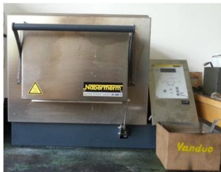
Figure.2.7.Furnace for tempering process
