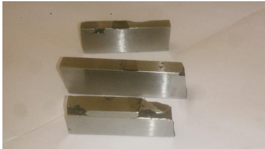
Figure.2.15 Samples after wear test and surface wear seen in this sample
