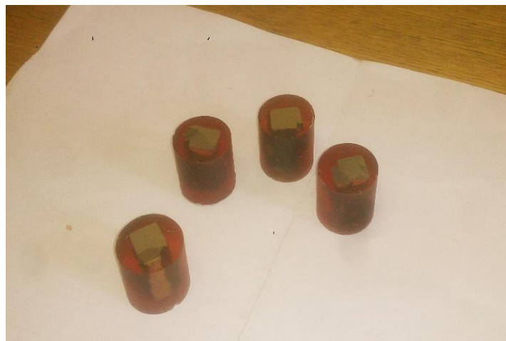
Figure.2.9 Prepared samples for microstructural analysis and etched
