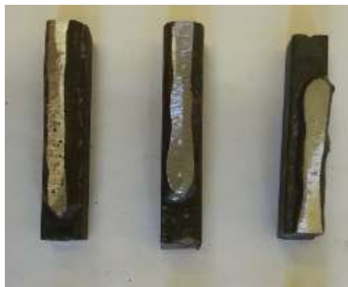
Fig. 3.2. Welding specimen's prepped and initial hardness tested
