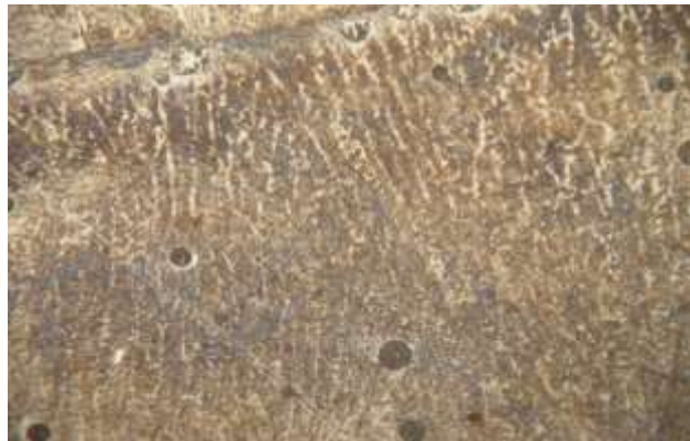
Fig. 3.15. Microstructure of Sample 05 after tempering. Magnification 200x
