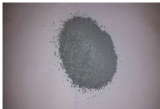
Fig. 2.3. Equal Mixture of Grounded Silicon Carbide (SiC) & Silicon Oxide (SiO)
