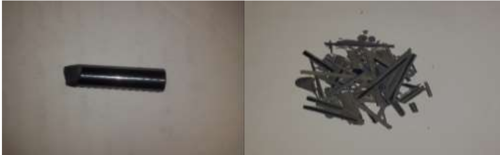
Fig. 2.4. Hard Material before and after annealing treatment
