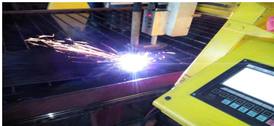
Fig 2.2 CNC plasma jet cutting
