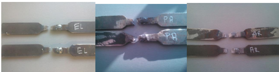
Fig. 3.10 Specimen's after tensile test
