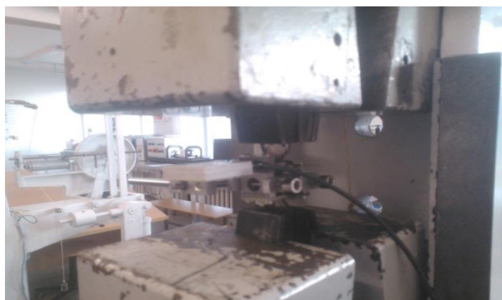
Fig 2.9 Displacement sensor attached to plate in order to measure displacements during stretching
