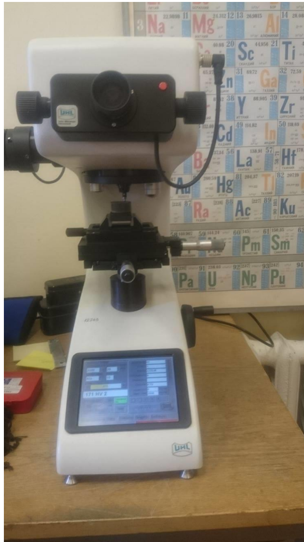
Fig. 2.21 VMHT micro hardness tester
