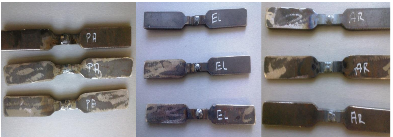
Fig. 2.7 Plates after welding. PA – 136 type, EL- 111 type, AR – 141 type.
