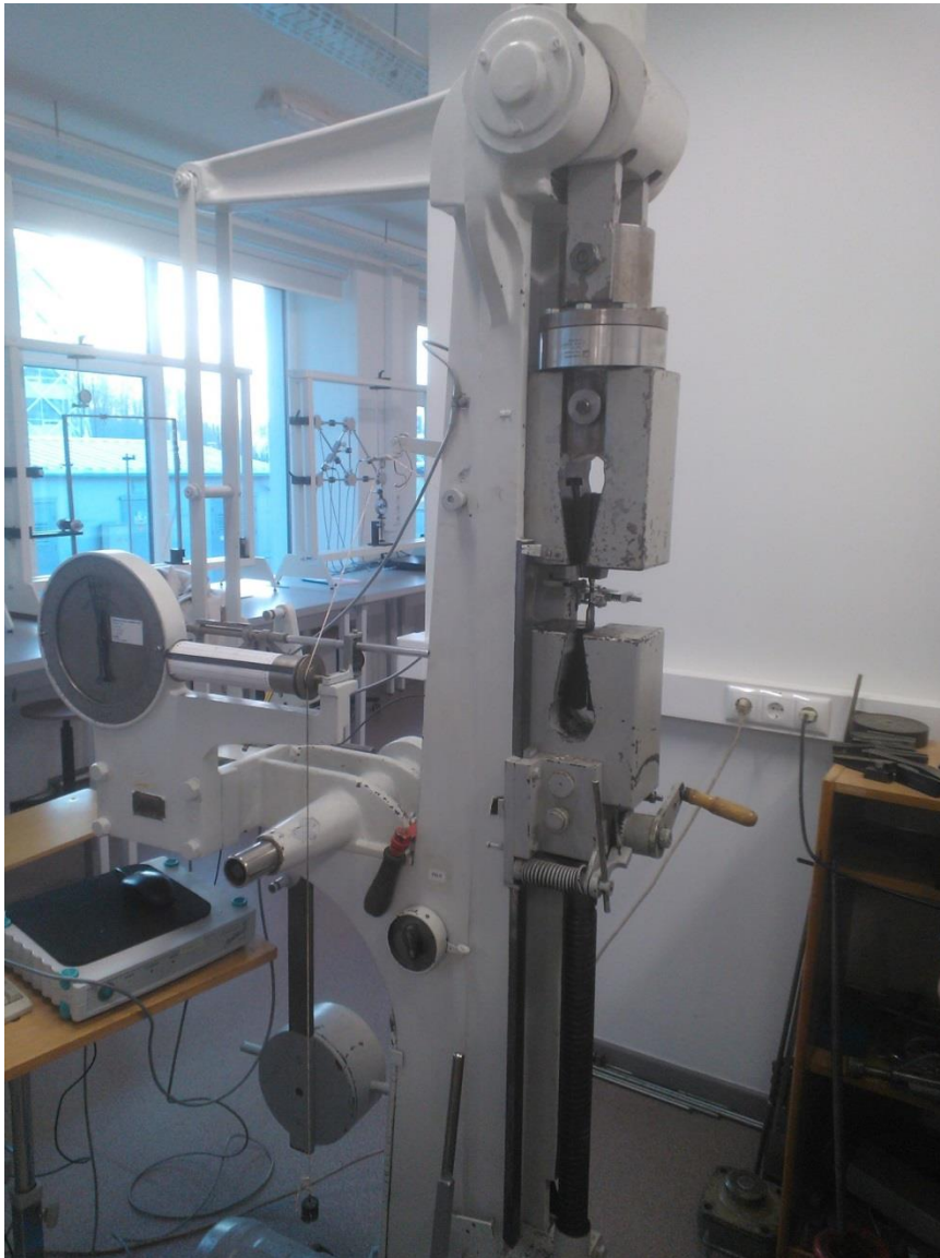
Fig. 2.18 Universal elektromechanical test machine. Maximum load capacity – 50 kN
