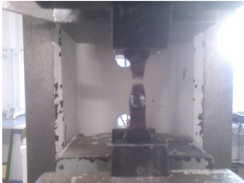
Fig. 2.8 Interrupted plate after stretching experiment
