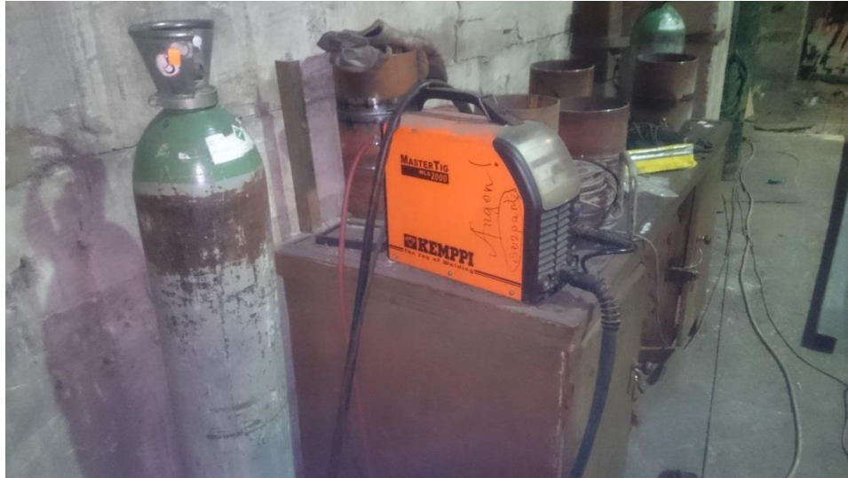
Fig. 2.14 For TIG and MMAW welding KEMPPi masterTIG MLS2000 were used
