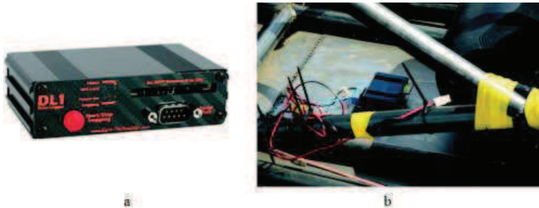
Fig. 5 Data collection device DL1 and its installation place in the buggy
