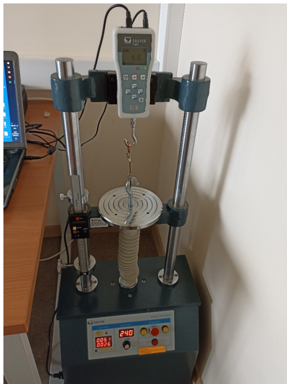
Figure 1. Test bench for mechanical testing; Sauter TVM 5000N230.
