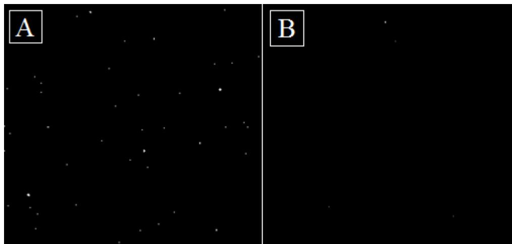
Figure 10. Threshold image captured with (A) unprotected camera and (B) protected camera.
