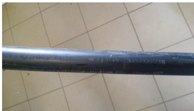
3 pav. Kabelis DRYREX AHXCMK-W TT 12 kV 1x120/16
