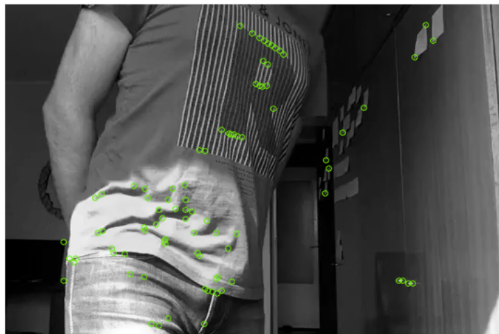
Figure 10 This image shows initial stage of Shi-Tomasi corner points
