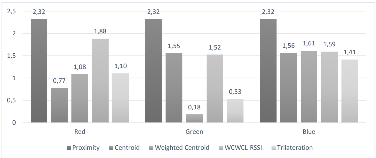
Figure 14. The histogram of calculation error for three beacons
