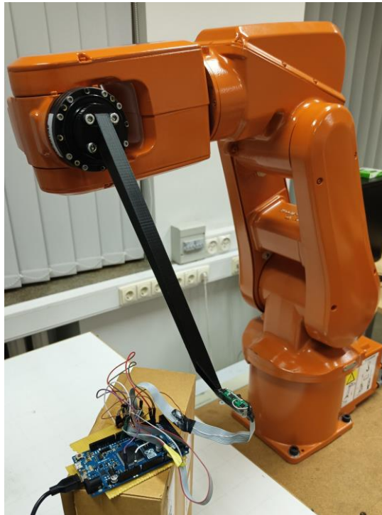
Fig. 3.16. Robotic arm with a sensor fastened to the custom mounting tool
