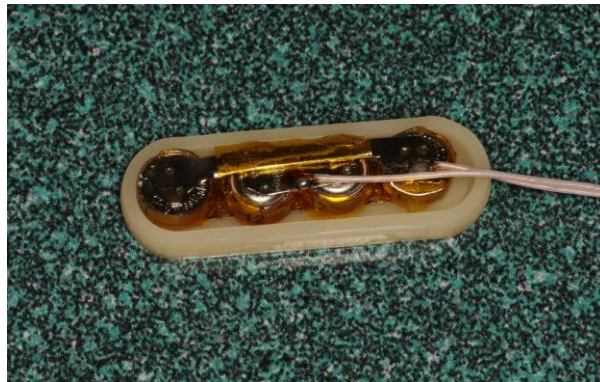
Fig. 3.13. Custom 3.1 V, 64 mAh battery pack
