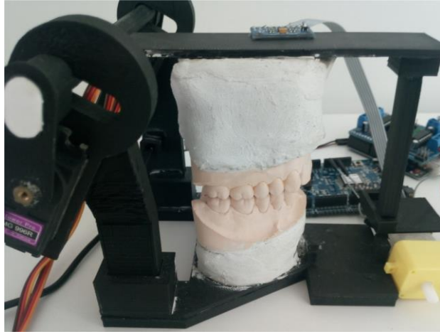
Fig. 3.4. Single-hinge vertical motion articulator with attached IMU
