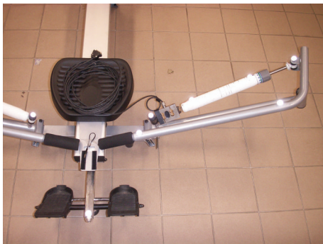
FIGURE 2: Location of the markers of 3D Qualisys mocap system on the rowing machine and HBM S9 type force sensor inserted between the hydraulic cylinder bottom end and the frame.
