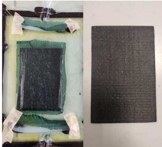
Figure 2: Specimen during the Vacuum Infusion and final product
