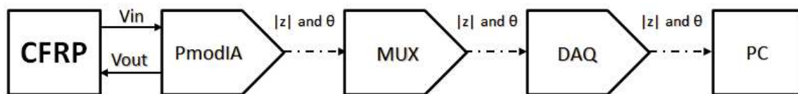
Fig. 5. The signal chain from CFRP under test to PC.
