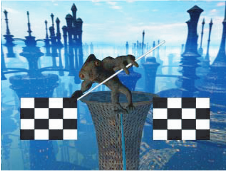
Figure 3.18: The players Avatar on a tightrope between two SSVEP checkerboards. The player must correct the avatar’s fall by focusing on the appropriate symbol [Lalor et al., 2005a]
