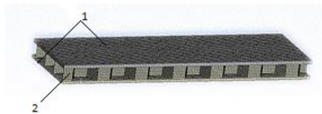
Figure 1. Model of sandwich with honeycomb core. 1 – woven glass fibre and polyvinylester resin composite facesheet; 2 - recycled paper hexagonal honeycomb impregnated in polyvinylester resin.
