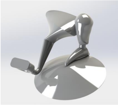
Fig. 3 The assembly of middle ear, performed in SolidWorks®2012 ([10])
