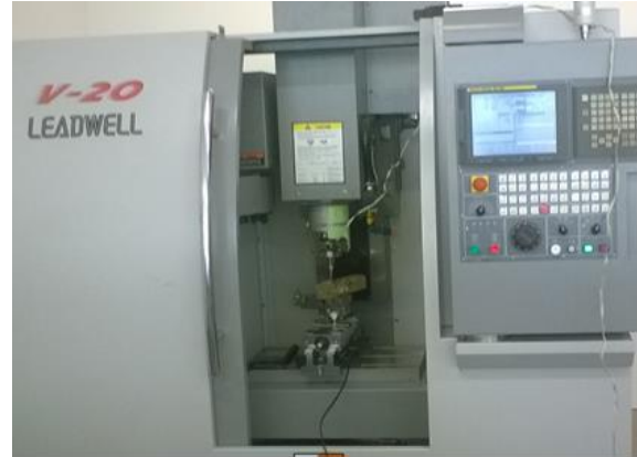
Fig. 1 “Leadwell” V20 CNC milling machine
