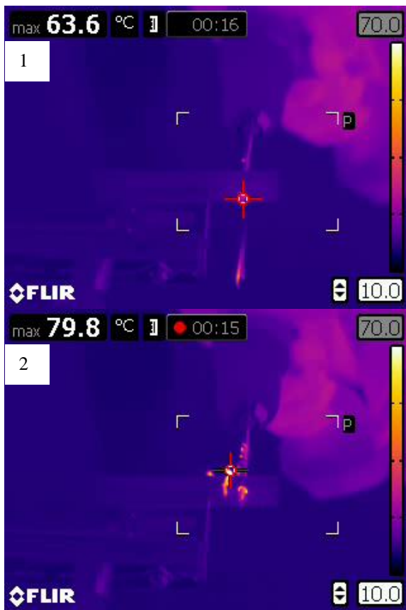
Fig. 11 Highest observed temperature: 1 – hole; 2 - chip
