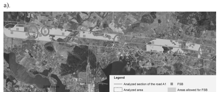
Fig. 11. a) The scheme of areas allowed for FSB construction and b) their overlapping with the existing FSBs (the removed FSBs are marked with red circles).
