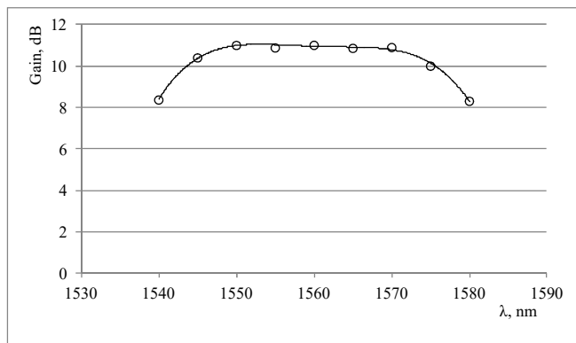
Fig. 3. The gain of RSOA as a function of wavelength.
