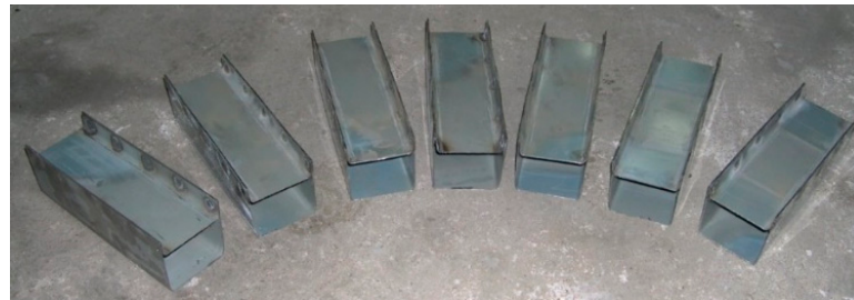
Figure 8. T1 specimens used in the quasi-static and dynamic experiments.
