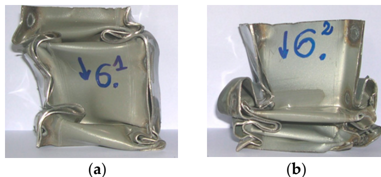
Figure 11. Specimens after the dynamic buckling experiments: specimen without broken spot-welded joints (a); specimen with two broken spot-welded joints (b).
