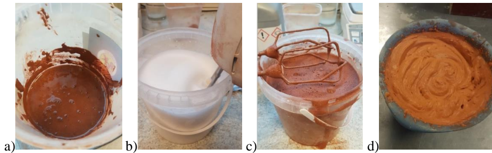
Figure 1. Foam preparation and casting process.
