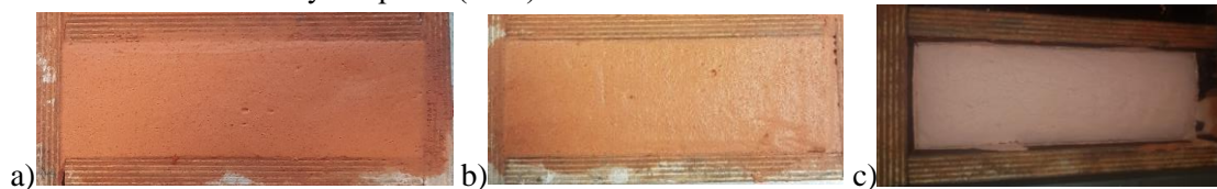
Figure 3. Casted samples of foamed geopolymers. a) without additives, b) with Portland cement additive, c) with H 2 O 2 foaming admixture.
