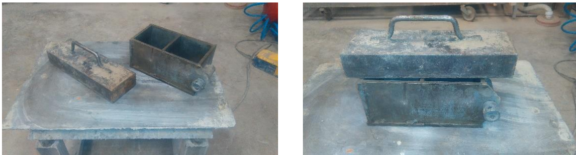
Figure 1. View of the test specimen compaction under the load of 11.63 kg (left: mould without load, right: mould with load).
