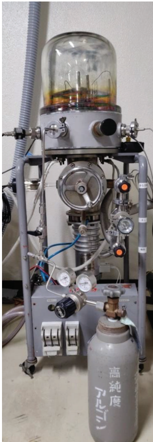
Fig. 2.3. Thermal evaporation system (a), sample holder with masks inside the chamber (b) and system schematics (c) where V1 – a valve between the chamber and the rotary pump, V2 – a valve between the rotary pump and the diffusion pump, V3 – a valve between the diffusion pump and the chamber
