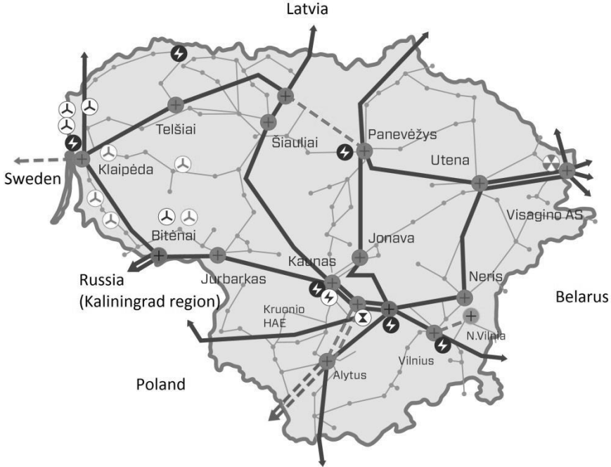
Figure 37. Lithuanian power transmission system (Courtesy of Litgrid).
