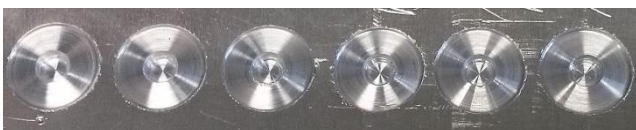
Fig. 3 Examples of stir spot welds
