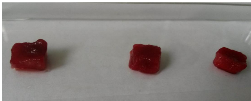
Fig. 3.38. Sponges No. 1-3 after the blood absorption test
