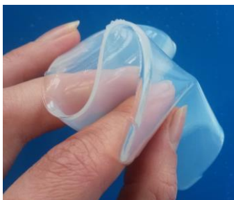
Fig. 3.3. Demonstrative flexibility of cellulose hydrogel
