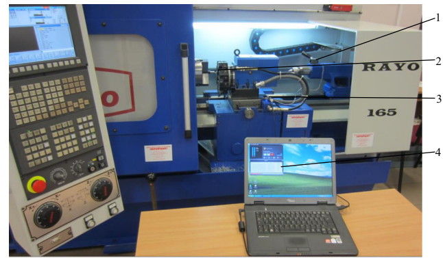
Fig. 15 Experimental setup for the diagnostics of acoustical signal during turning: 1 microphone of the acoustical measurement device, 2 zone of turning process, 3 controller of acoustic signal, and 4 PC with the acoustic signal analysis program
