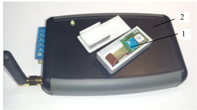
Fig. 7 General view of the electrical energy harvester with the energy accumulation, wireless transmitter (1) and diagnostic signal receiver (2)
