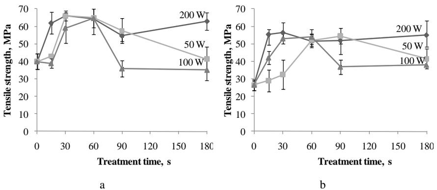
**Fig. 5.** Influence of low-pressure nitrogen plasma treatment parameters on the cotton (a) and flax (b) yarn reinforced PLA composites tensile strength
