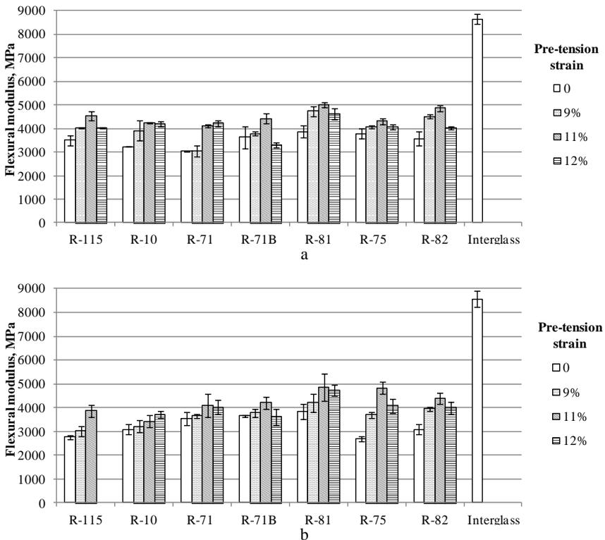
**Fig. 13.** The influence of pre-tension on the flexure modulus of biocomposite in warp (a) and in weft (b) directions
