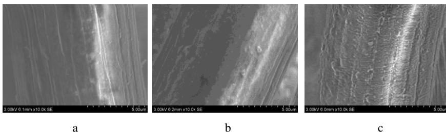
**Fig. 3.** SEM images of untreated cotton fiber (a), after exposure at 50 W for 180 s (b) and after exposure at 200 W for 180 s (c)
