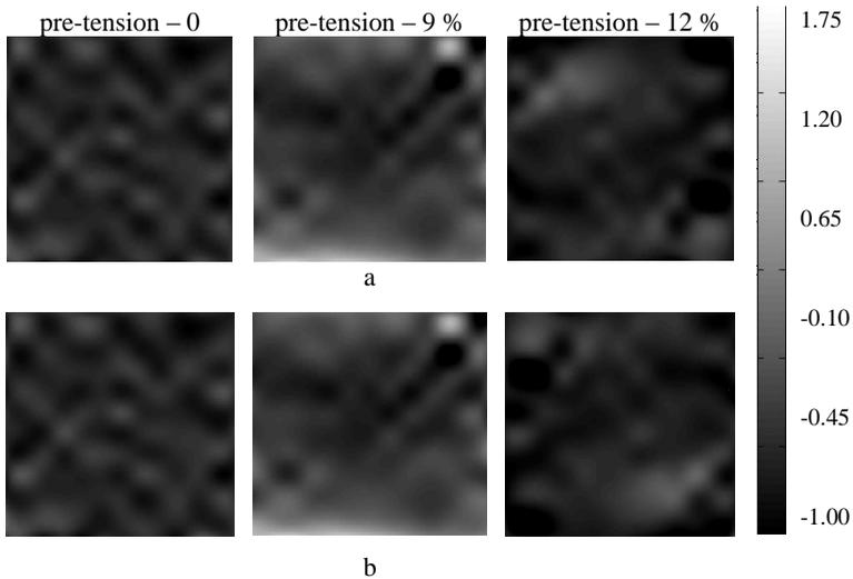
**Fig. 14.** The deformation field in fabric R71 during pre-tension: (a) warp and (b) weft directions
