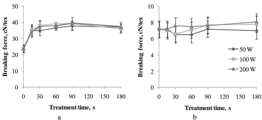
**Fig. 4.** Influence of low-pressure nitrogen plasma treatment parameters on the cotton (a) and flax (b) yarn tensile strength
