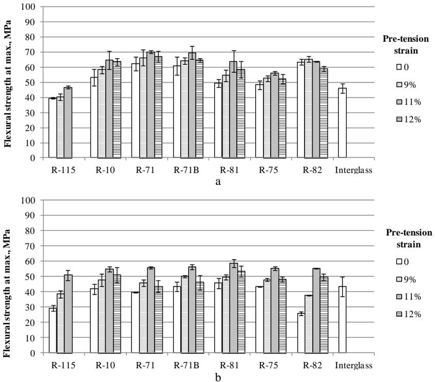
**Fig. 12.** The influence of pre-tension on the flexure strength of biocomposite in warp (a) and in weft (b) directions
