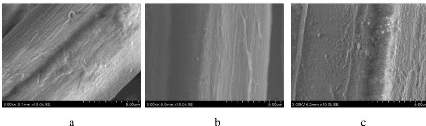
**Fig. 2.** SEM images of untreated flax fiber (a), after exposure at 50 W for 180 s (b) and after exposure at 200 W for 180 s (c)
