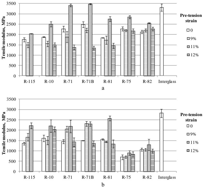
**Fig. 11.** The influence of pre-tension on the tensile modulus of biocomposite in warp (a) and in weft (b) directions
