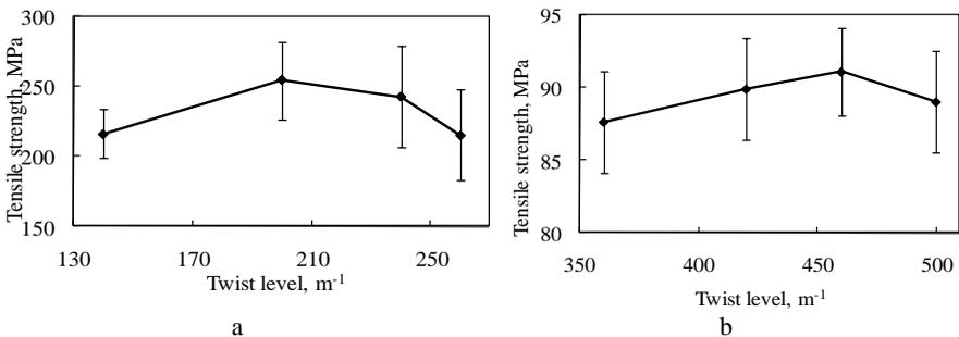
**Fig. 8.** The influence of twisting level on natural fibers tensile strength: a – 105 tex flax; b – 70 tex cotton
