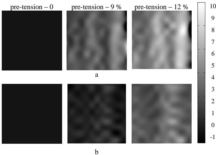
**Fig. 10.** The deformation field in fabric R71 during pre-tension: (a) warp and (b) weft directions
