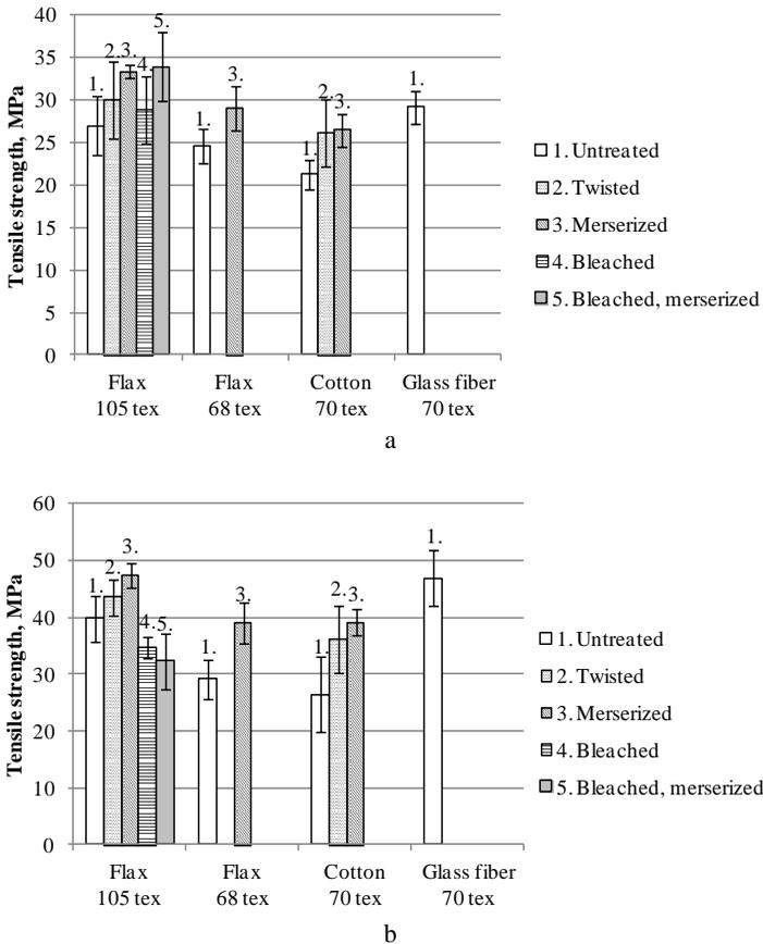
**Fig. 1.** Influence of fiber treatment methods on the tensile strength of UP (a) and PLA (b) composites
