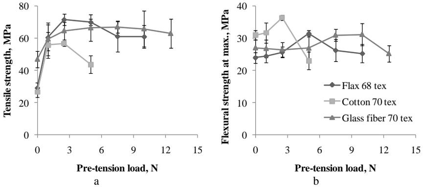
**Fig. 7.** The influence of pre-tension load upon the tensile (a) and flexural (b) strength of composites
