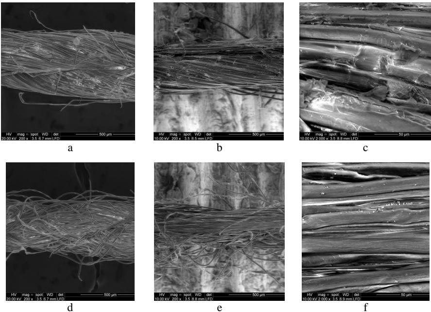
**Fig. 6.** SEM micrographs of flax (a – c) and cotton (d – f) fibres: a, d – un-stretched; b, e – pre-tensioned (magnification 200×); c, f – pre-tensioned (magnification 2 000×)
