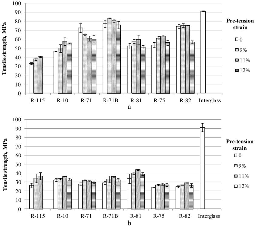
**Fig. 9.** The influence of pre-tension upon the tensile strength of flax/UP composite in warp (a) and in weft (b) directions
