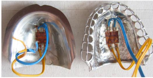
Fig. 1.25 Strain gauges attached to SPIF denture samples [50]
