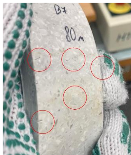
Figure 9. Patterned artificial cast stone after bending test at 170 °C (cracks are marked in red).
