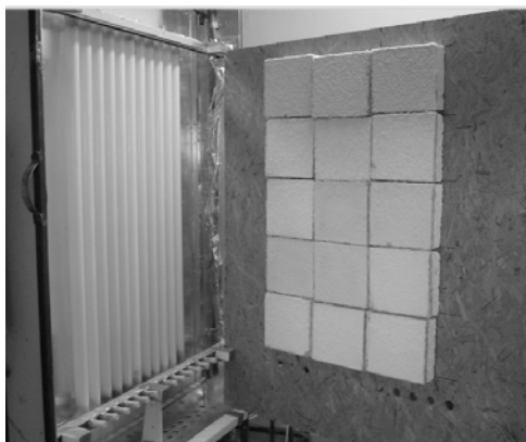
Fig. 1. The prepared ETICS samples for the laboratory testing in the UV climatic chamber
