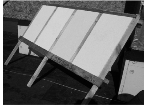
Fig. 2. The ETICS panels (1000×500×50 mm) for the natural ageing placed on the wooden test rack
