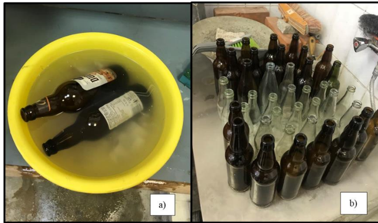
Fig. 25. Cleaning process of the Glass: a) Clean the papers with hot water. b) Wash inside and outside of glasses
