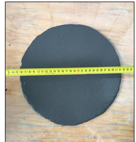
Fig. 40. Measuring the cement paste circle
