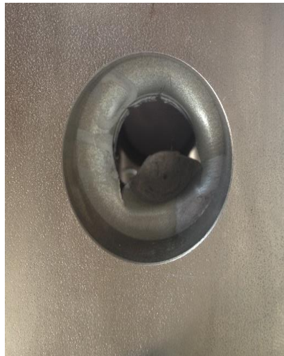
Fig 4.3 fracture of the specimen in cupping test experiment
