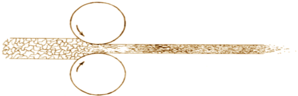
Fig 1.1 schematic representation of rolling process[15]
