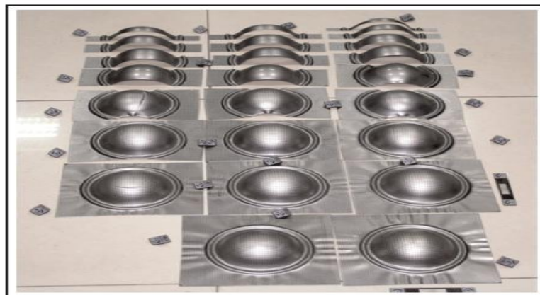
Fig 2.10 specimens for the Nakazima experiment.[14]
