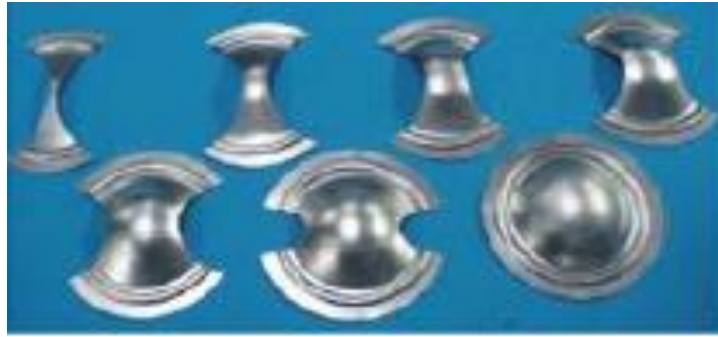
Fig 2.7 specimens for the Marciniak experiment [14]
