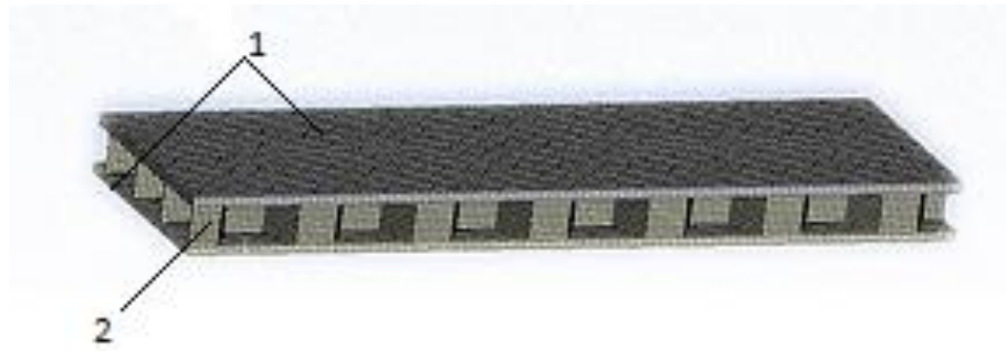
Fig 3.4. Model of sandwich with honeycomb core.1 – woven glass fibre and polyvinylester resin composite facesheet; 2 - recycled paper hexagonal honeycomb impregnated in polyvinylester resin
