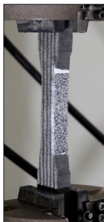
Figure 4 : ASTM D638-14 test setup
