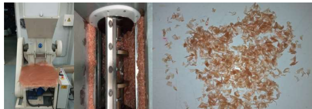
Figure 2. Vacuum bags shredding process
