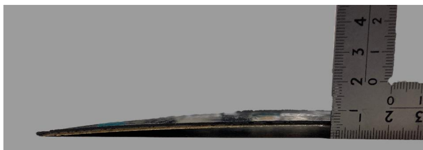
Figure 4 [0^{\text{CFRP}}_4/0^{\text{NFC}}_4] After drying for 3 days
