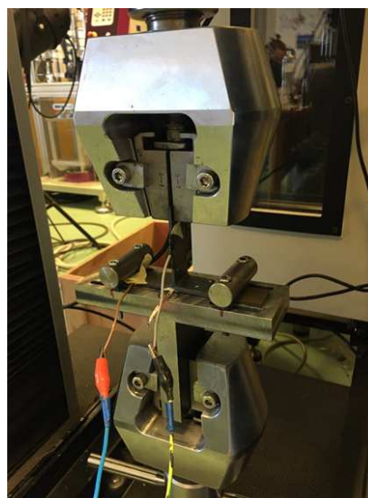
Figure 3. Special experimental setup for t-joint debonding.
