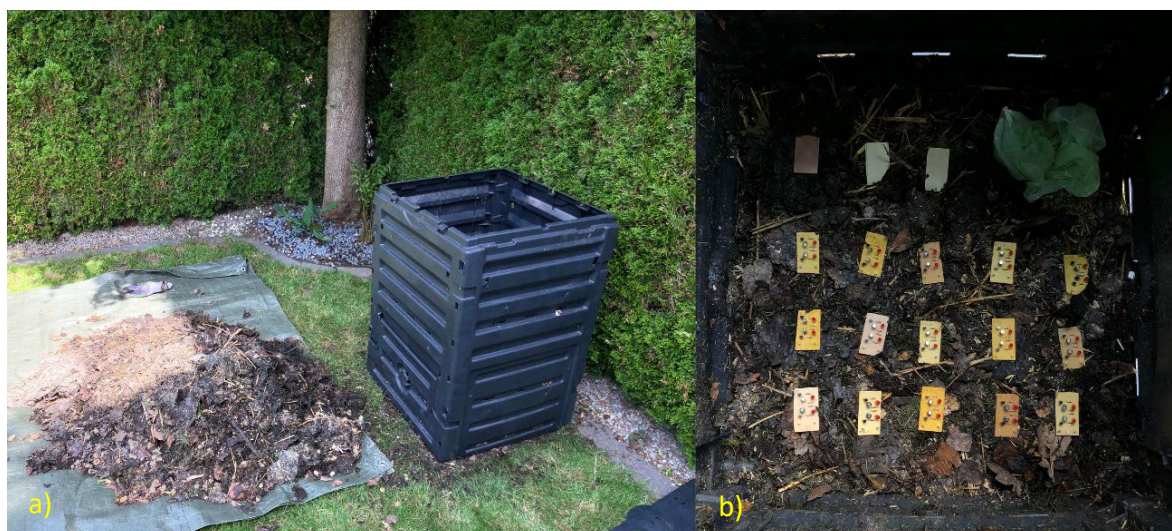
Figure 4. a) Compost bin with organic filling, b) CNF, BC and epoxy PCBs placed inside the compost.
