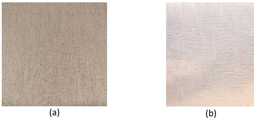
Figure 1. Unidirectional flax fabric (a) and unidirectional glass fabric (b).
