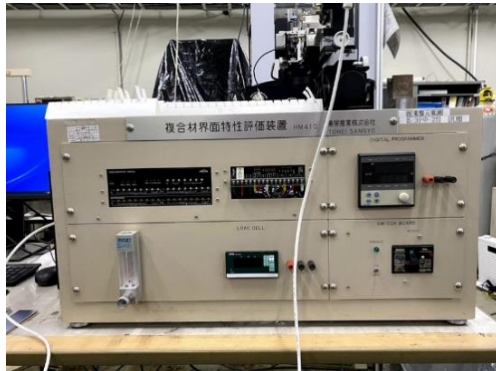
Figure 5. Test machine for micro-droplet tests.
