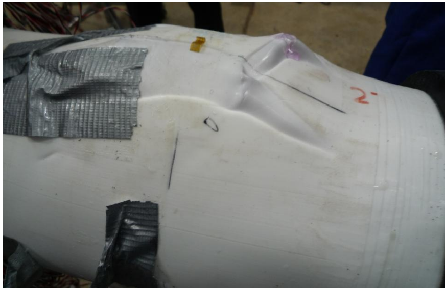
Fig. 7 Photograph of the failed hydrostatic pressure test sample. A debonded strain gauge is visible on top.
