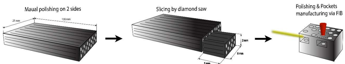
Figure 1: Micromechanical specimen preparation and workflow (not to scale). Left : The top (25x100 mm 2 ) and side (25x2 mm 2 ) faces are manually polished. Middle : micromechanical sample is sliced. Right : The sample is mounted on an SEM stub (not shown) and a pocket is milled via FIB.
