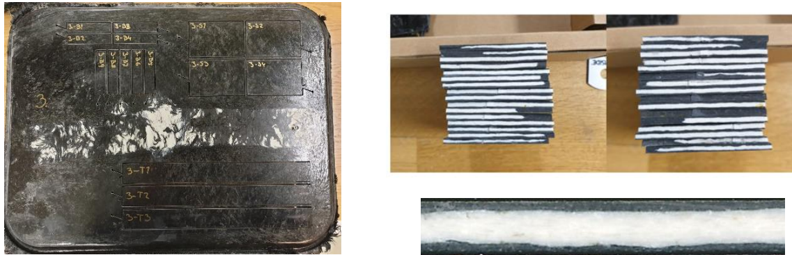
Figure 2: (a) One of the hybrid plates (b) side view of a stack of samples from the hybrid plate
