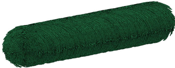
Figure 2: Generated spun yarn model with twist of 75 \text{ m}^{-1} and fiber length distribution
