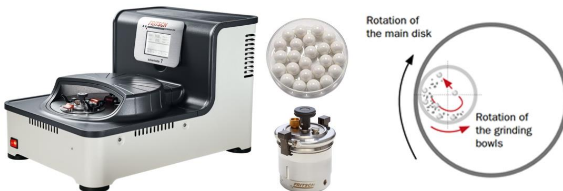
Figure 2. Milling of carbon particles ( https://www.fritsch-international.com/sample-preparation/milling/planetary-mills/details/product/pulverisette-7-premium-line/ )
