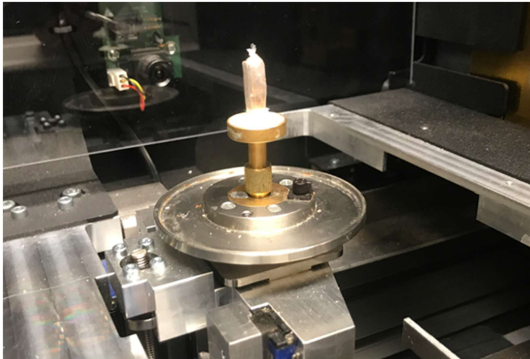
Figure 2. A stack of wooden cubes in the X-ray micro-CT, encapsulated in plastic foil with salt equilibration at given levels of relative humidity.
