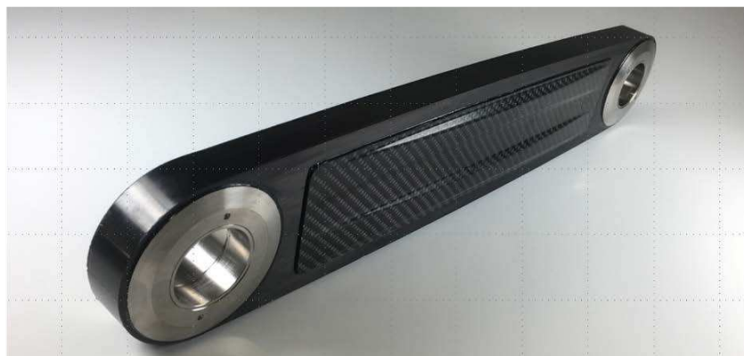
Figure 7 : Complex test specimen of the strut structure with novel CFRP-titanium hybrid design in overall dimensions of 515 mm x 36 mm x 95 mm, representing a scale of approximately 1:2 compared to the reference
