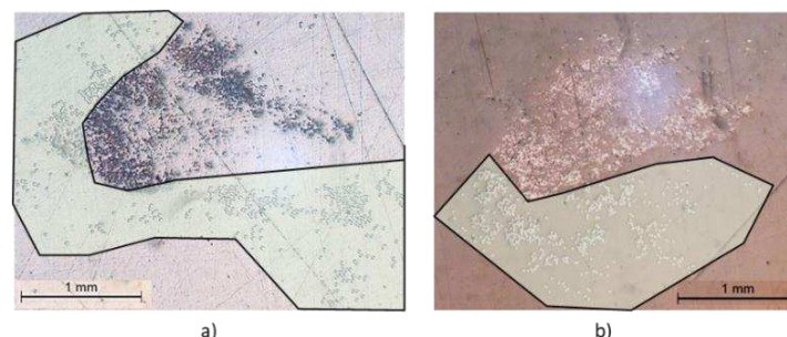
Figure 4. Optical microscopy images of PPS/CF a) commingled and b) hybridized yarns.
