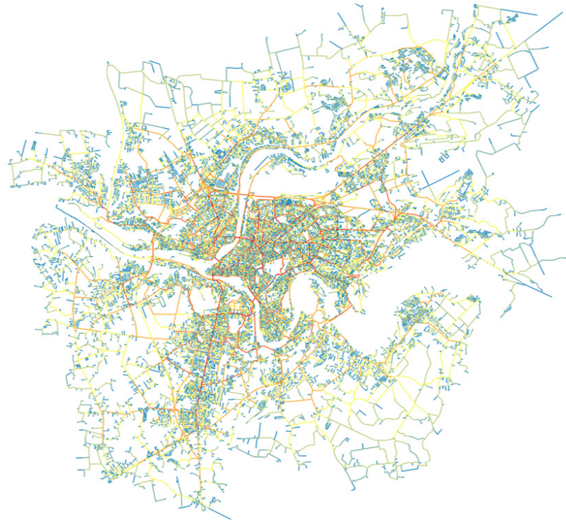
Figure A3. Kaunas, Choice within radius 5000 m. Red indicates high and blue low numerical values.
