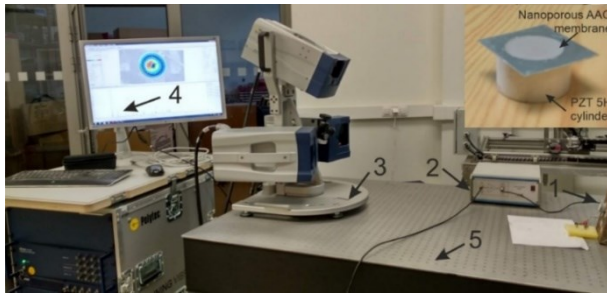
Fig. 4. 17 Experimental setup of the 3D scanning vibrometer for the actuation of the fabricated nanoporous membrane: cylindrical PZT-5H actuator (1), linear voltage amplifier ( FLC P200 ) (2), 3D vibrometer PSV-500-3D-HV (3), a computer interface with analysis software (4), anti-vibrating table (5)
