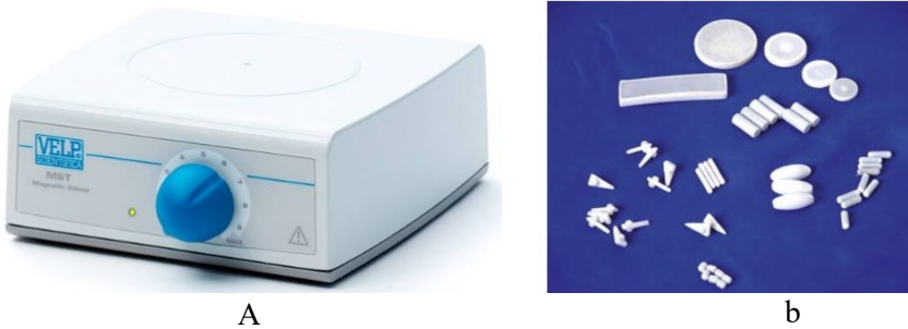
Fig. 2. 11 Magnetic stirrer (a), and magnetic stirrer bar for mixing the electrolyte (b) [153]
