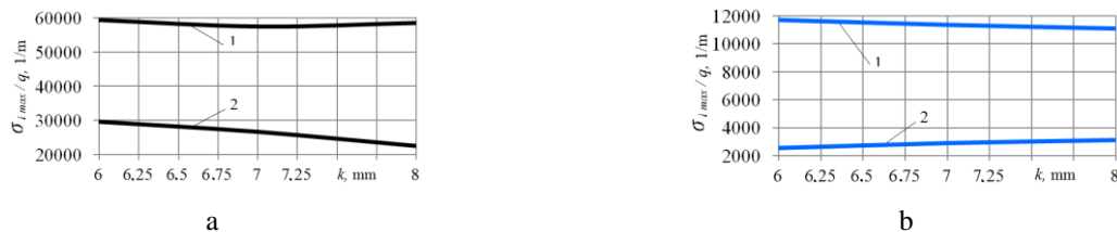
Figure 4. The largest relative tension intensity dependence from the corrugated grid sheet thickness in different materials of the beam is, when k = 6 mm, 7 mm, 8 mm: a - in the corrugated bridge; b - in wooden girders (1 - at the ends of the beam 2 - at the middle of the beam)
