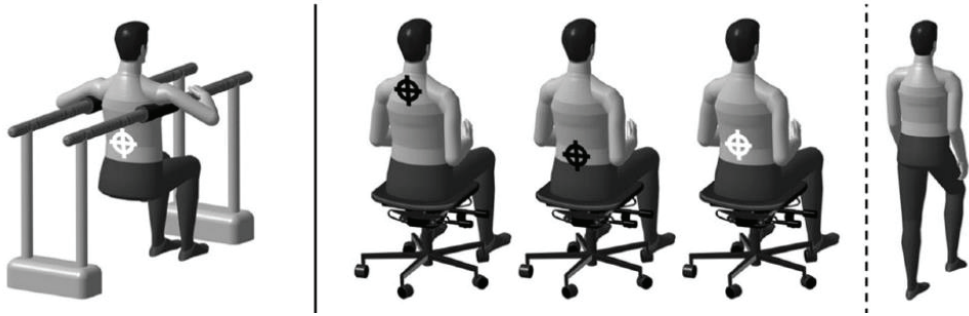
Figure 7. Physiological motion axis during free sitting, on different types of chairs and when in walking [50]
