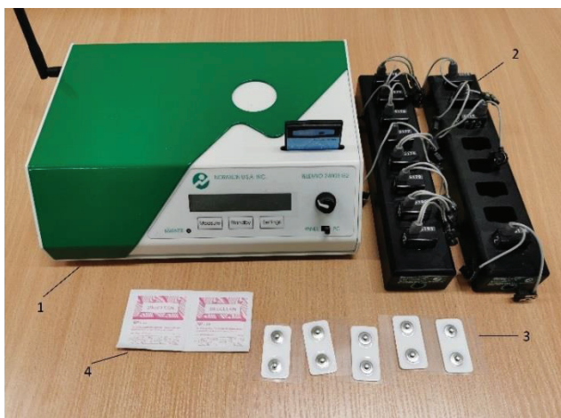
Figure 20. The setup of EMG system: electromyograph (1), channels (2), electrodes (3), alcohol wipes (4)
