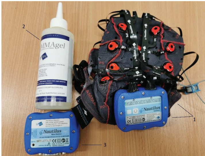
Figure 27. Set up of the EEG measurement: wireless electroencephalograph with cap (1), gamma gel (2), base station (3)
