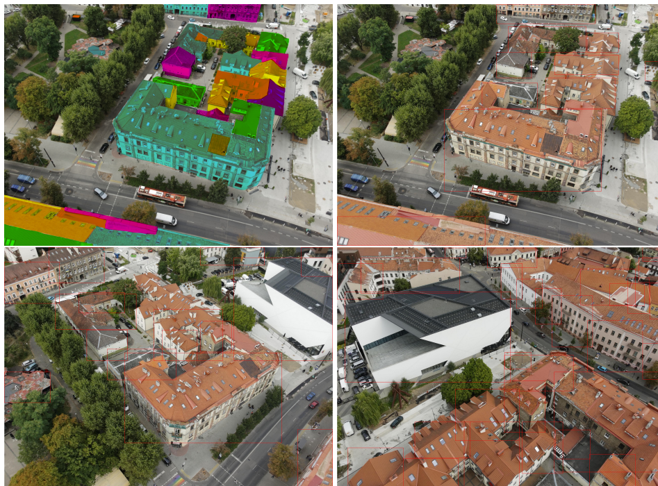
Figure 13. UAV camera images showing G⊙ center and M⊙ museum area at different angles. The red mark indicates a detected façade shape. Color highlights show assigned segment masks.
