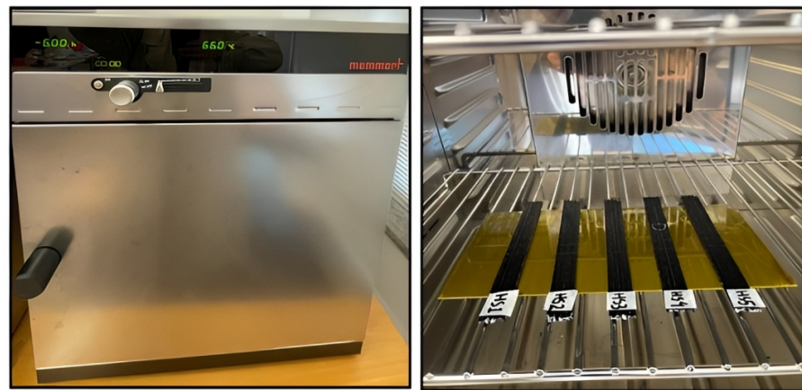
Figure 2. An air-circulated oven for hot temperature treatment.
