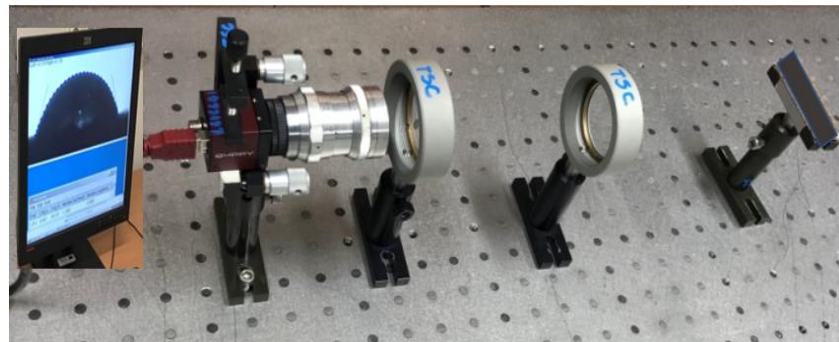
Figure 1. A contact angle measurement setup.
