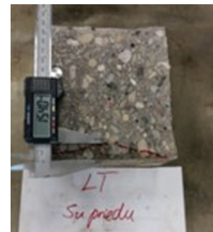
Fig. 4. Depth of water penetration of concrete samples.
