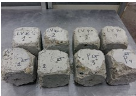
Fig. 3. Concrete samples after 100 days in ammonium sulphate solution (148 g/l).
