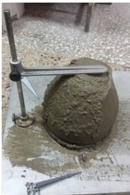
3.19 pav. Betono mišinio su priedu BLIVS/PROOF (Vincent's Polyline) slankumo bandymas
