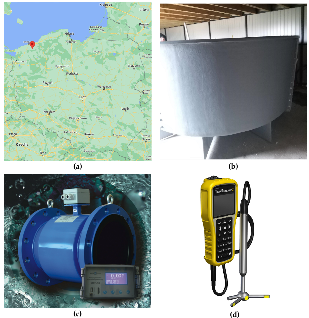
Figure 1. Location of the RAS fish farm and the equipment used in experiments: (a) location of Gdynia, Poland shown on the map; (b) fish tank type SDK-RT 29-68 mounted on site; (c) electromagnetic water-flow meter MTF-10 (source: http://www.mtfplow.pl accessed on 13 September 2022); (d) SonTek FlowTracker2 Handheld-ADV (source: https://www.yssi.com/flowtracker2 accessed on 13 September 2022).
