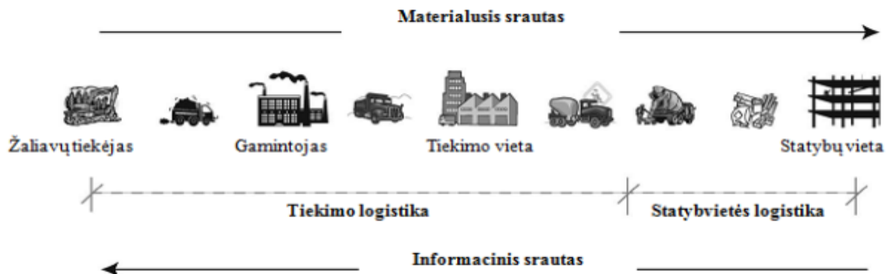
8 pav. Statybų logistikos funkcijos (A project manager`s level of satisfaction in construction logistics. Canadian Journal of Civil Engineering, nr. 30, 6p, 2003)
