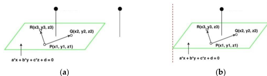
Figure 7. Plane limits: (a) calculates the distance to all points, (b) discards the points that are outside the limits of the current plane.
