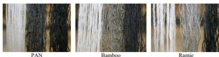
Figure 1. Example of modified fibres (from left to right): before treatment, after the first cycle of treatment, after the second cycle of treatment.
