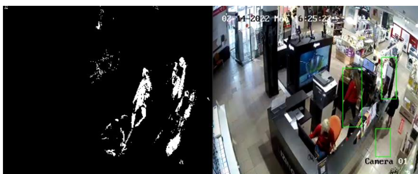
Figure 5. An example of moving object detection using MOG2 algorithm.
