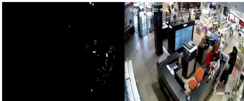
Figure 4. An example of image processing when movement is not detected.
