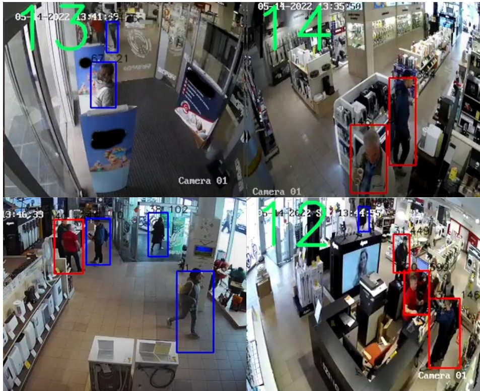
Figure 13. Examples of live object tracking the store.
