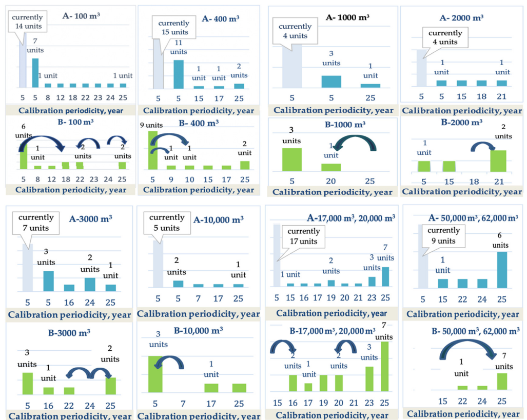
Figure 6. Calculated calibration intervals, using standard method (diagram A) and modified method (diagram B). Arrows show the changes in the results obtained by the modified calculation method compared to the standard calculation method.
