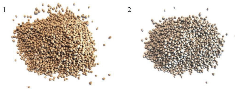
Fig. 3.7. NPK 11-10-16+MgO+S+B fertilizer granulated under industrial conditions: 1 – without biomass ash; 2 – with biomass ash
