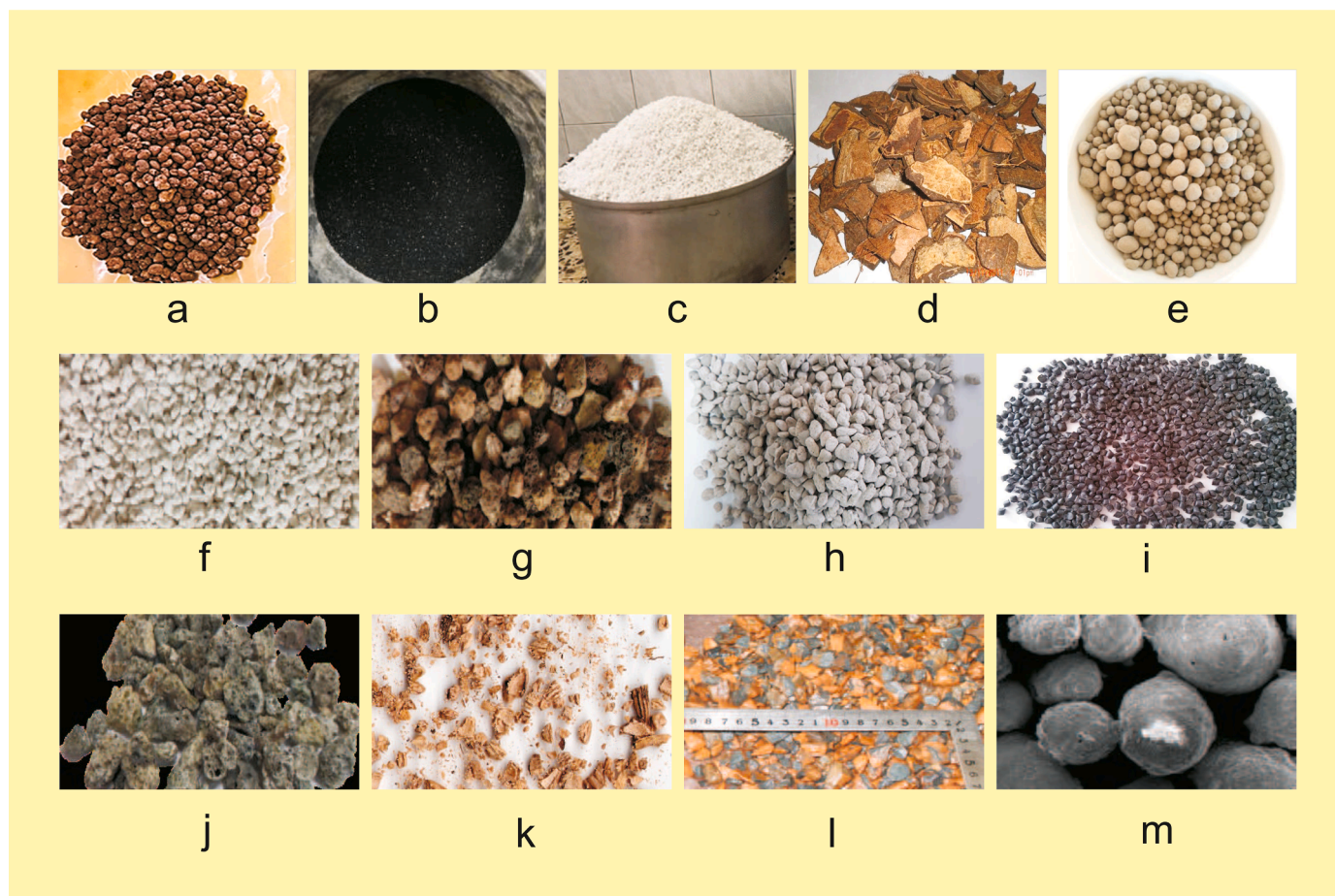
Figure 2. The shape of different types of LWA: a. expanded clay (Nahhab and Ketab, 2020); b. rubber (Hossain et al., 2020); c. EPS (Medher et al., 2021); d. coconut shell (Poongodi and Murthi, 2020); e. fly ash aggregate (Güneyisi et al., 2016); f. perlite (Dolatabad et al., 2020); g. scoria (Dolatabad et al., 2020); h. pumice (Agwa et al., 2020); i. recycled plastics (Faraj et al., 2021); j. POC (Feen et al., 2017); k. olive kernel shells (Cheboub et al., 2020); l. expanded shale (Wu et al., 2009); m. expanded glass (Spiesz et al., 2013).
